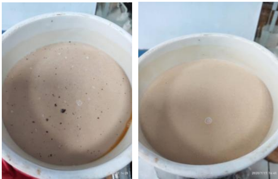
Figure 1. Comparison of sodium oxalate precipitation from seed after three precipitation cycles
